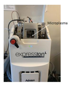
Liquid sampling-atmospheric pressure glow discharge (LS-APGD) microplasma integrated with an Advion Compact Mass Spectrometer (CMS) for at-reactor elemental analysis.
